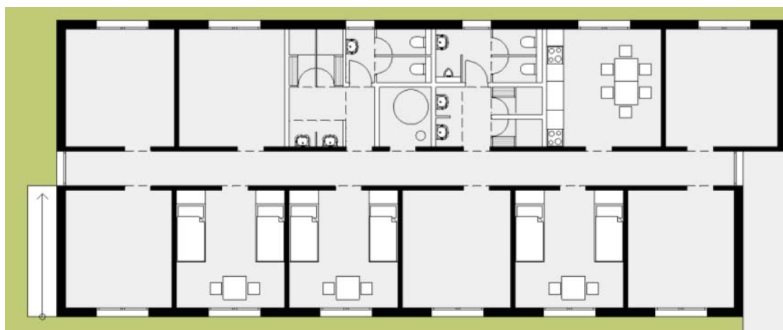
Munich: Floor plan, two-room apartments with communal kitchen and sanitation area
