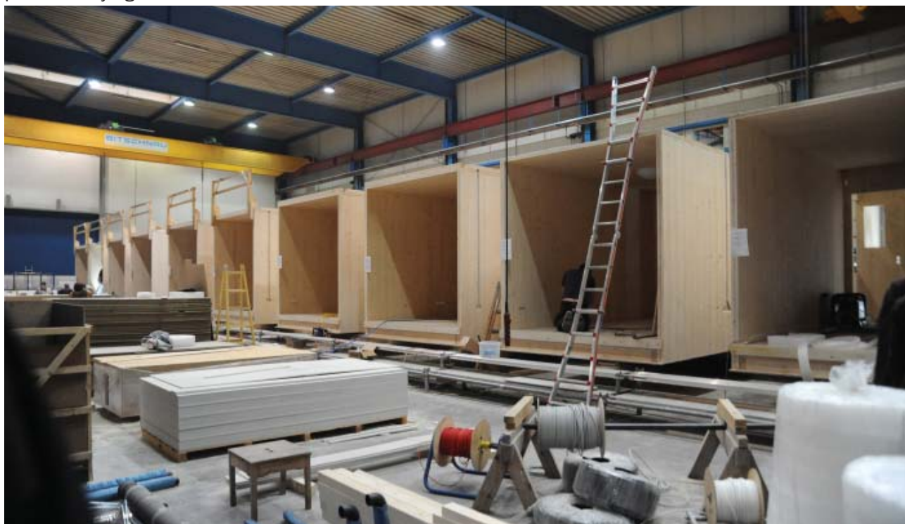
Producing the modules in Vorarlberg / Photo: © MOSAIK Architekten BDA
