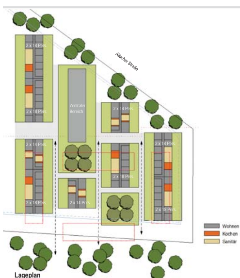
Munich: Site plan and diagram of modular building method
